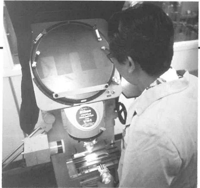
Tool inspection at Kras Asia being carried out under a precision projector.
